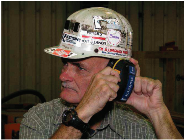
Figure 3 — Worker adjusting the volume control on the QuickFit device to set his hearing threshold prior to inserting an earplug.
