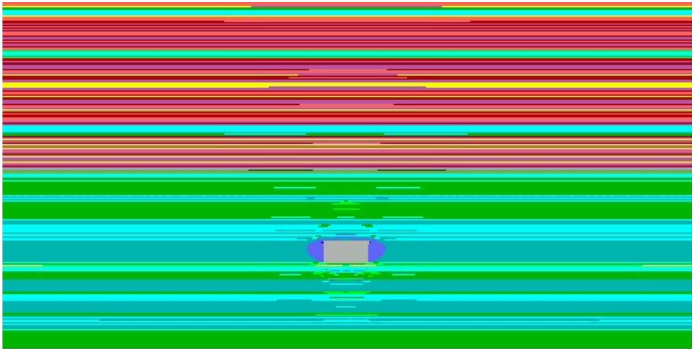
Fig. 5. Initial horizontal stresses. Warm colors indicate high horizontal stress in stiffer layers, and cool colors indicate low horizontal stress in less stiff layers. The future entry is shown at center.
