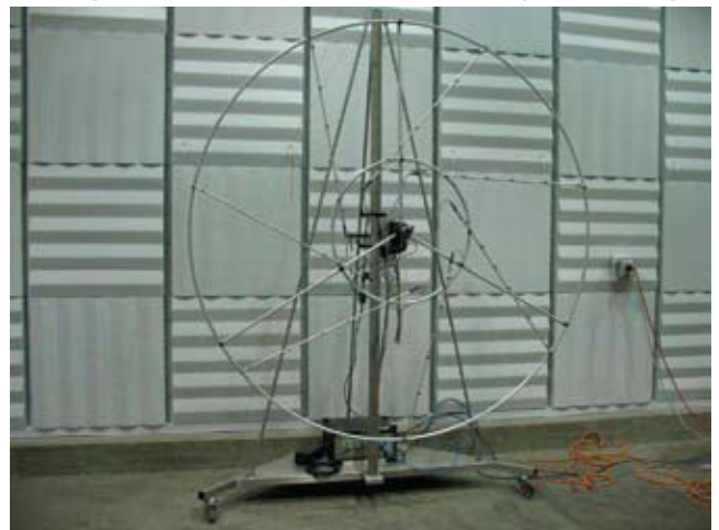
Forty-two channel acoustic beamforming wheel array.
