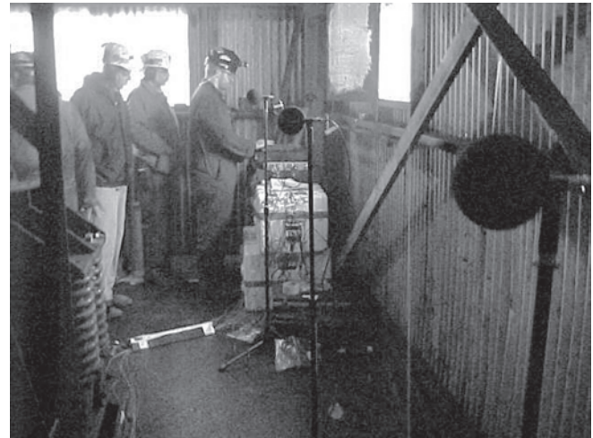
Figure 5 — Data acquisition equipment location and microphones along left side of Screen 169.
