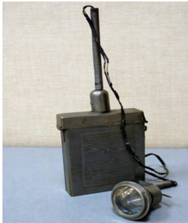
Figure 1. The Edison Electric Cap Lamp (circa 1915) from the NIOSH collection of mine illumination. Image courtesy of New South Associates.
