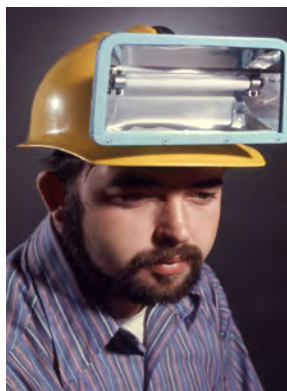
Figure 4. The development of a fluorescent cap lamp enabled the evaluation of this new technology. Source: NIOSH mining photo archive.
