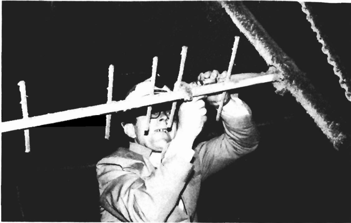
FIGURE 3.19. VIEW OF YAGI ANTENNA INSIDE THE PORTAL SHOWING SEVERAL MONTHS' ENCRUSTATION OF LIMESTONE DUST AND SMOKE PARTICLES ON THE ANTENNA RODS. THE ANTENNA VSWR WAS NOT READABLE WITH 2.5 WATTS FORWARD POWER AND PERFORMANCE EVIDENTLY WAS NOT DEGRADED.
