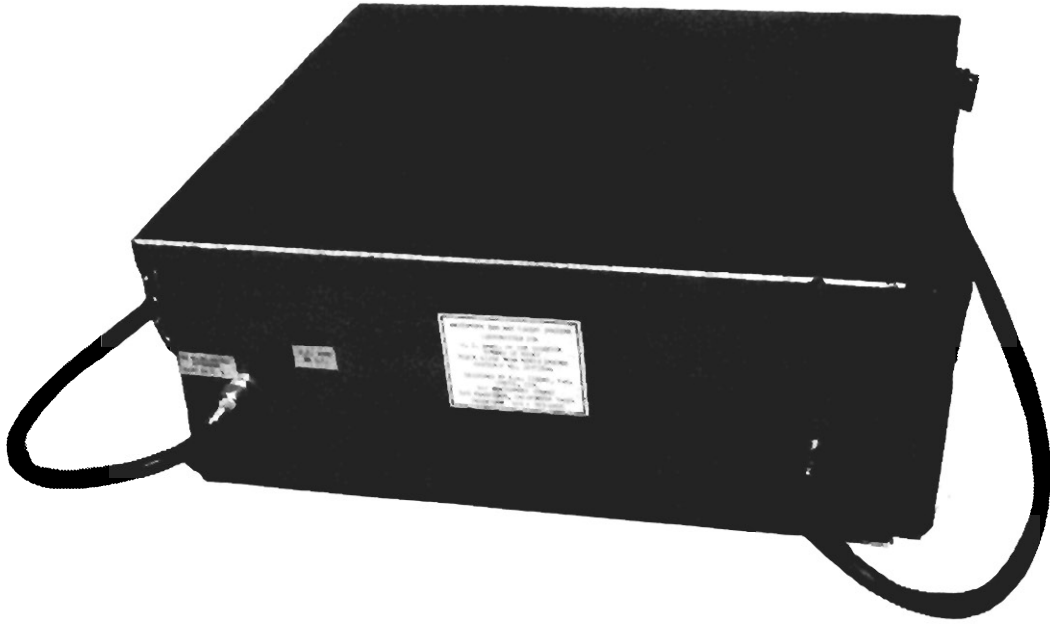
FIGURE 3.11.A PROTOTYPE TWO WAY UHF SIGNAL BOOSTER IN NEMA CLASS 4 ENCLOSURE
