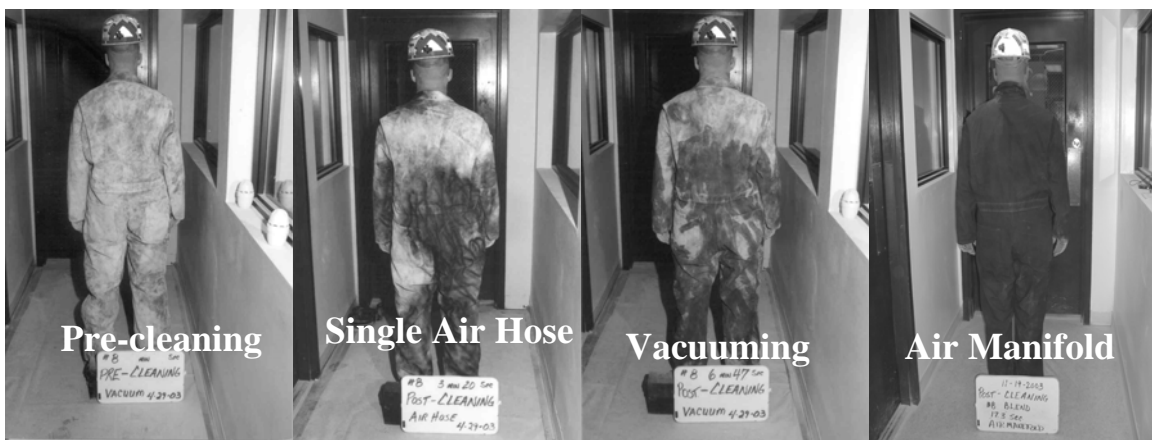
Figure 6. Effectiveness of various cleaning methods.
