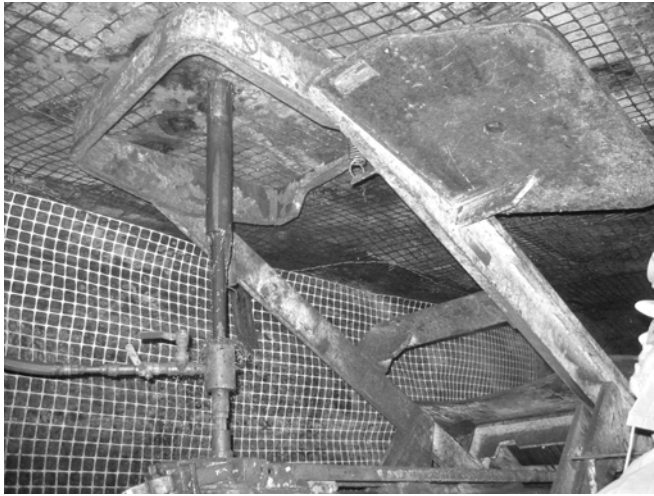
Figure 4. Bolt overcoring equipment; NX core barrel, EW drill rod, water swivel and hex steel adaptors.
