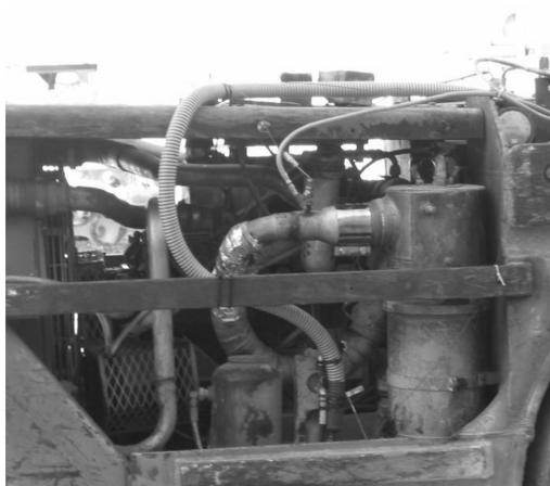
Figure 1. ArvinMeritor DPF system installation.
