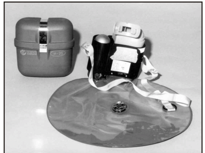
Figure 6.—Cased and uncased Ocenco M-20 self-rescuer.
