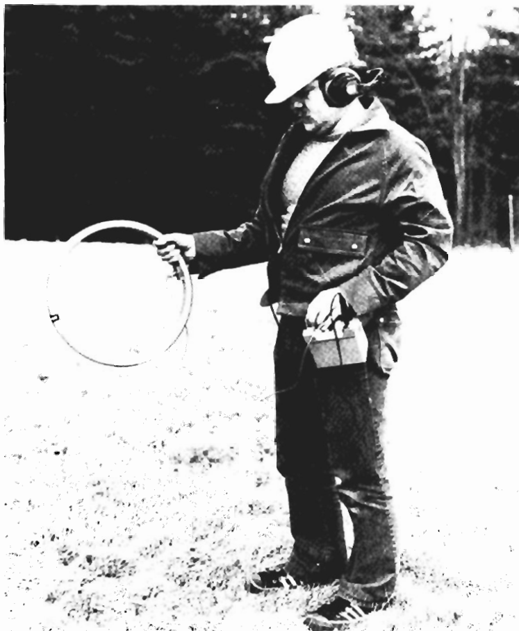
FIGURE 4. - Portable ULF EM receiver and loop antenna in use at a simulated mine disaster.
