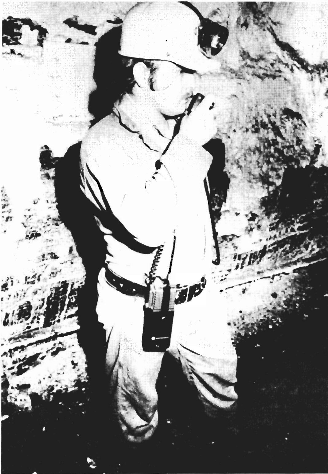
FIGURE 7. - Miner using intrinsically safe handy talkie unit.
