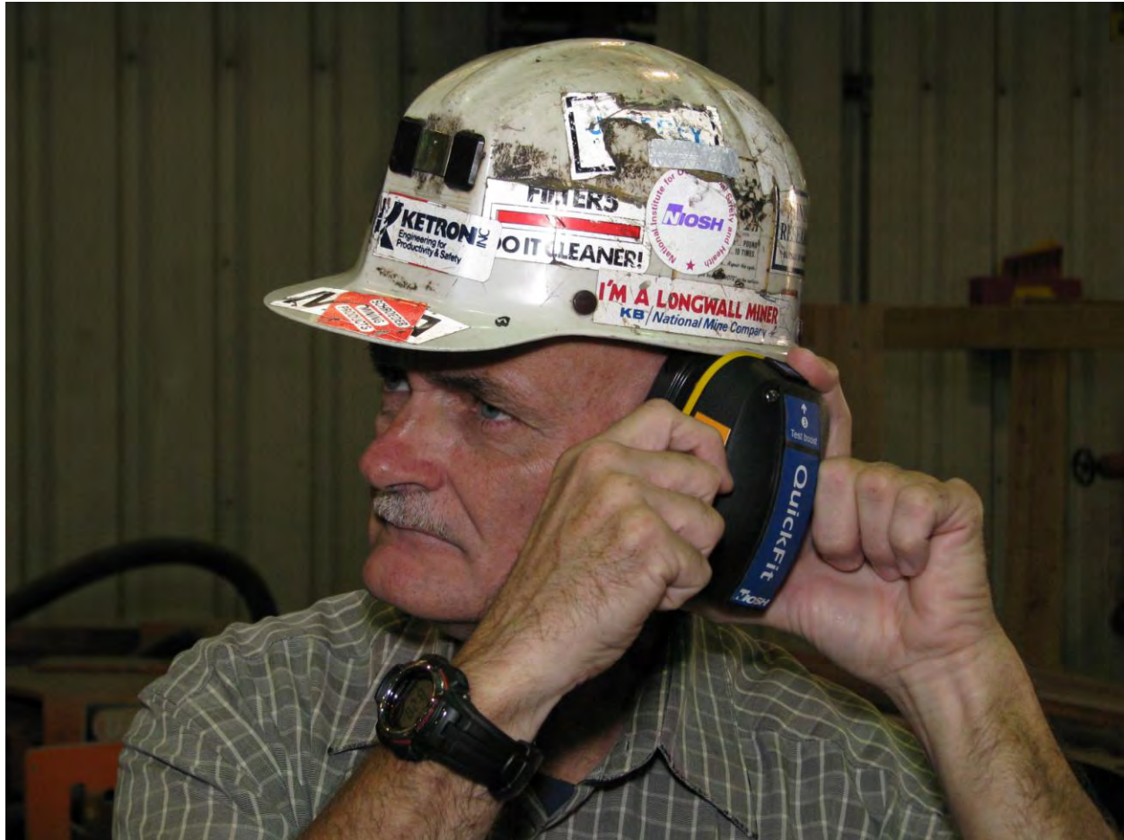
Figure 4. Testing earplug fit with the NIOSH QuickFit device.
