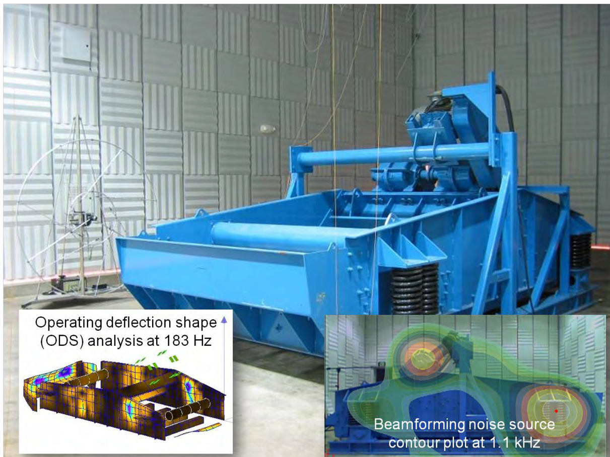
Figure 1. Vibrating screen assembly inside the NIOSH hemi-anechoic chamber next to microphone phased array used for noise source identification via the beamforming technique. Insets show results of operating deflection shape analysis and beamforming analysis.
