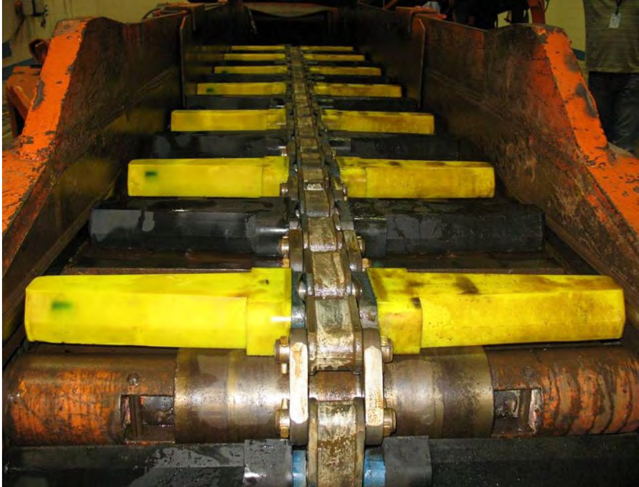
Figure 2. NIOSH-developed coated flight bars on a continuous mining machine conveying system.
