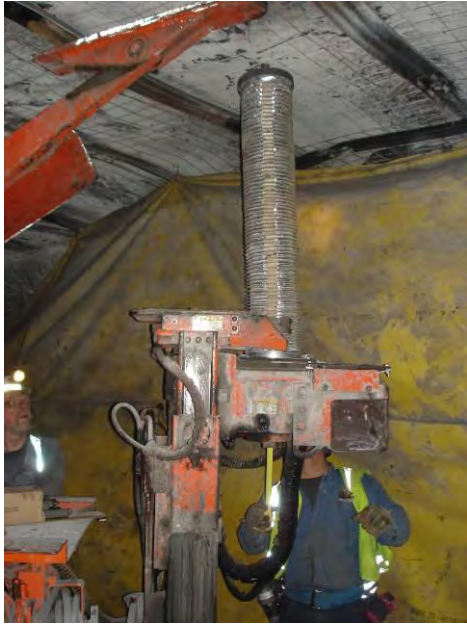
Figure 3. NIOSH-developed collapsible drill steel enclosure to control noise on roof bolting machines.
