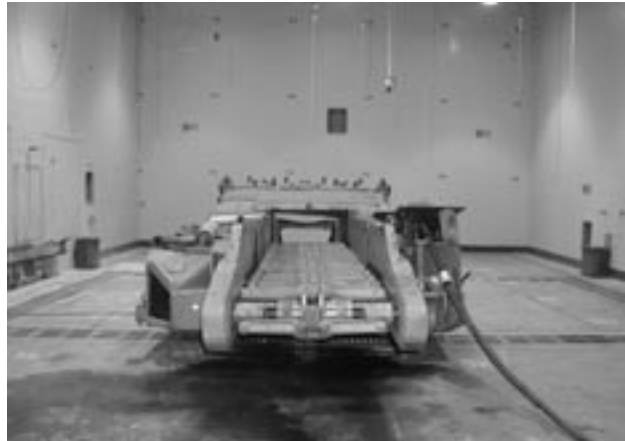
Figure 5. Continuous mining machine in the reverberation room at the NIOSH-PRL.
