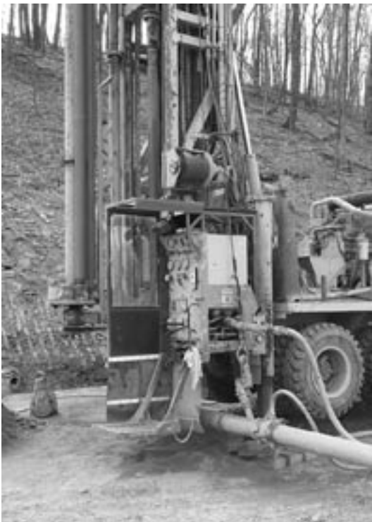
Figure 4. Partial cab installed on an air-rotary drilling rig.
