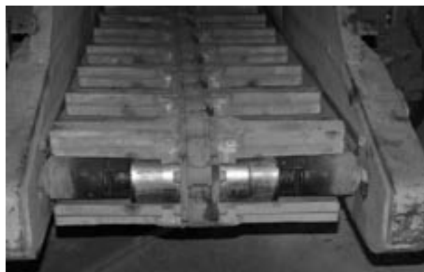
Figure 3. Coated flight bars on a continuous mining machine in an underground coal mine.
