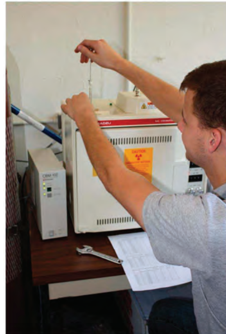
Figure 2 — In-house gas chromatographic analyses of gas samples for determination of SF 6 concentrations.
