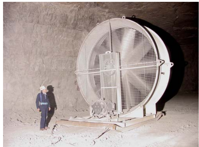
Figure 10. 3.65 m (12 ft) propeller fan used for regional airflow studies.
