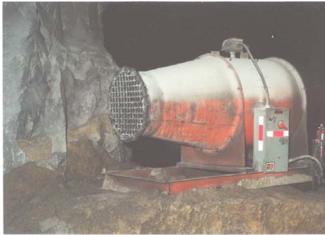
Figure 1. 0.91 m (36 in) vane-axial fan with 0.58 m (23 in) reducer.
