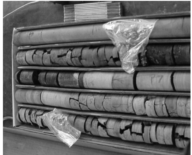
Figure 6. Core separated into specimens for point load testing at different time intervals. Bag samples were tested for moisture loss.
