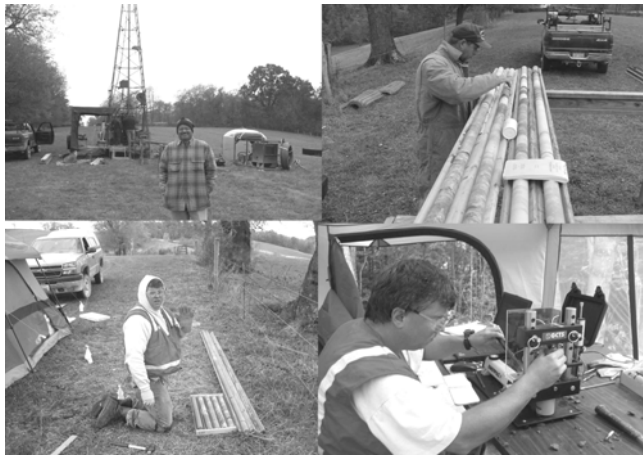
Figure 4. Pictorial overview of stages of fieldwork at both drill sites; clockwise from top left: (a) Diamond rock core drilling at site 2; (b) geologic logging of core runs at site 2; (c) axial PLT-UCS measurements of core specimen at site 1; (d) boxing of core runs in labeled core boxes made of wax permeated cardboard at site 2.
