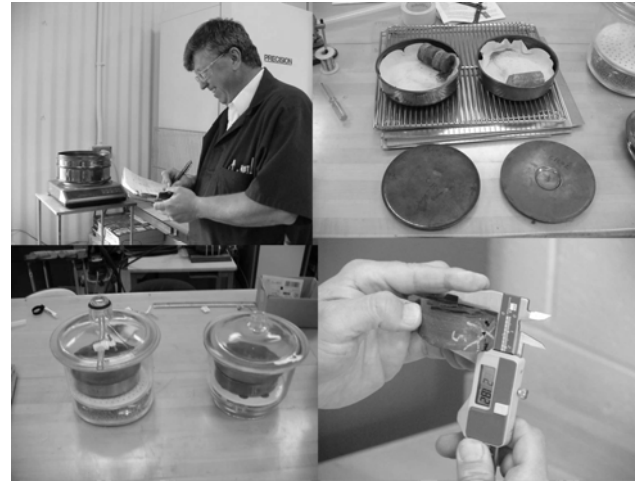
Figure 5. Pictorial overview of test stages of moisture content tests; clockwise from top left: (a) weighing of container and core specimen prior to precision oven drying; (b) post-dried core specimens in containers; (c) post-test measurements of bulk volume of core specimen; (d) vacuum desiccators with core specimen in weighing containers for specimen cooling without moisture loss prior to post-dried specimen weighing.
