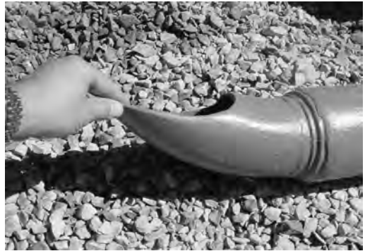
Figure 3. Directional elbow for bulk fill placement.
