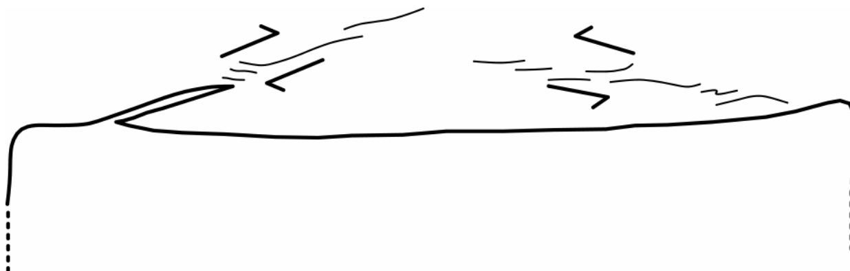
Figure 1.— Representative cross section showing fracture patterns in halite roof (modified from Terrill and VandeKraats 1997: figure 6).
