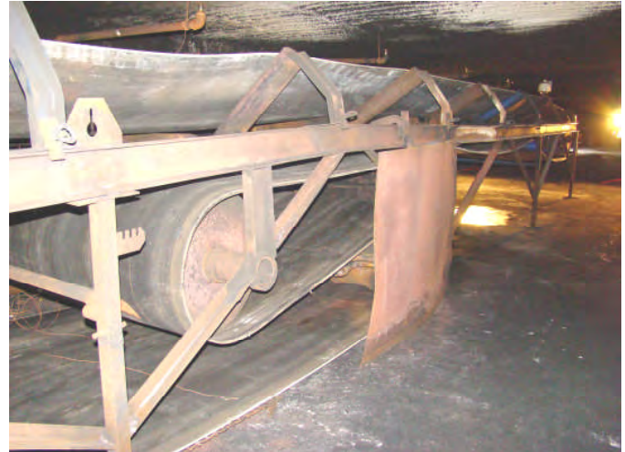
Figure 2. Fifty-five gallon drum as drive roller.
