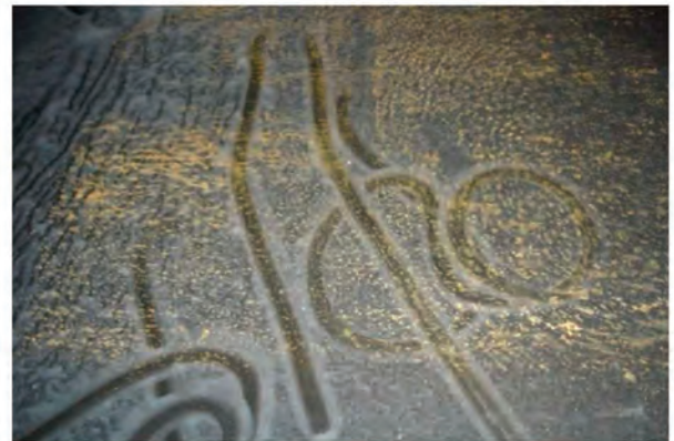
Figure 6 — Barricade II coating on top conveyor belt after sprinkler application test.
