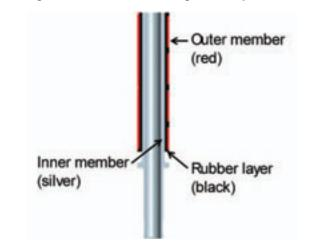
Rockwell C to improve resistance to cracking. Reducing the hardness increases the fracture toughness, reducing the brittleness and likelihood of the device cracking. The prototype in the current tests combines the design modification of a 30-cm (12-in.) cylinder length, inner and outer molded bonds, and 35 Rockwell C hardness.
