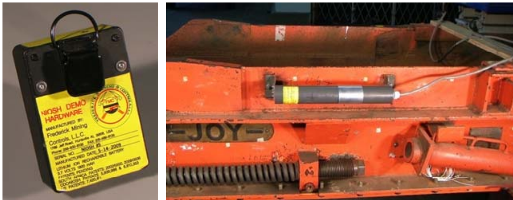
Figure 8: Electromagnetic PAD and field generator used for prototype system.
