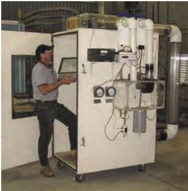
This 72-cubic-foot enclosed cab test stand was used in the filtration system experiments.
