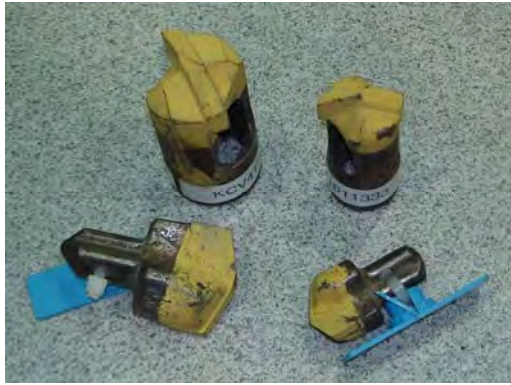
Figure 2 - Drills bits; vacuum (top), wet (bottom), 2.54 and 3.49 cm
