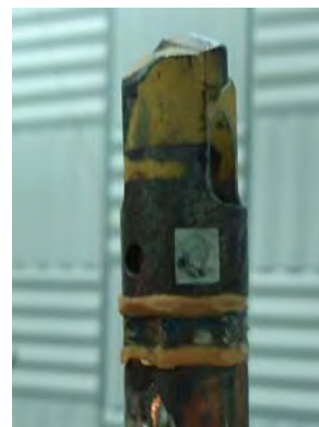
Figure 10 – Bit isolator with 60 Shore D urethane coating
