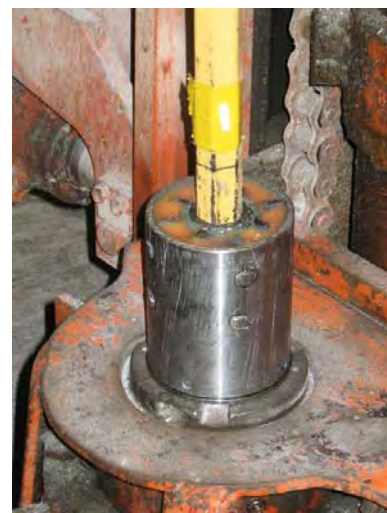
Figure 17 - Chuck isolator 2, 45 Shore A polyurethane filled
