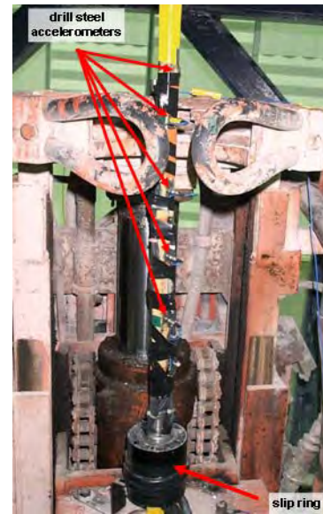
Figure 3 - Drill steel accelerometers and slip-ring assembly
