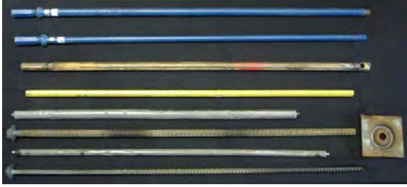
Figure 1 - Drill steels (round & hex), bolt plate, resin and resin type roof bolts, shown for 2.54 and 3.49 cm bit drilling and bolting
