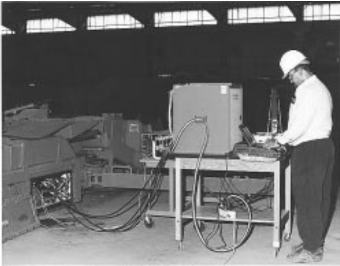
Fig. 1. Measuring motor-start waveforms on a 950-V continuous mining machine.
