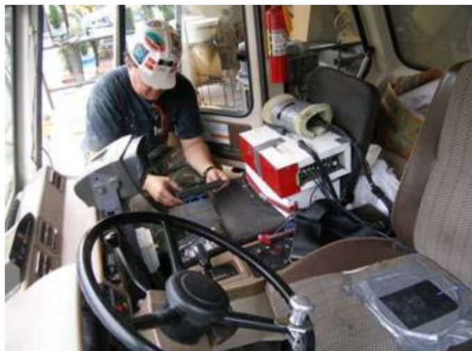
Figure 1. Instrumentation installed to collect WBV exposures for haulage truck operators. Tri-axial accelerometers are placed on the seat (seat pad) and on the vehicle frame next to the cab window.
