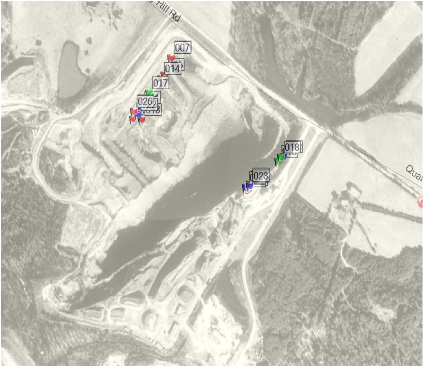
Figure 3. Marker flags overlaid on aerial photograph of aggregate stone quarry derived from GPS data. The numbered flags show locations where peak accelerations exceeded 10 \text{ m/s}^2 .
