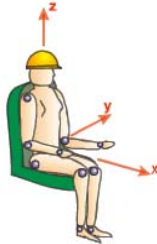
Figure 2. Vibrations levels are measured along the orthogonal x, y and z axes or vectors.
