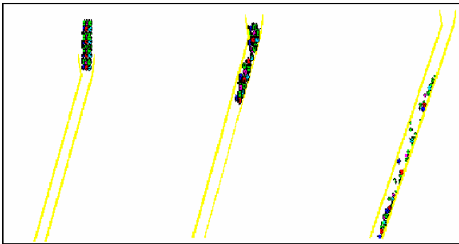
Figure 3.—WM2D simulations of flow in ore pass. Left: Particles just entering an inclined ore pass; middle: particles after being dumped into ore pass; right: particles have fallen a certain distance.
