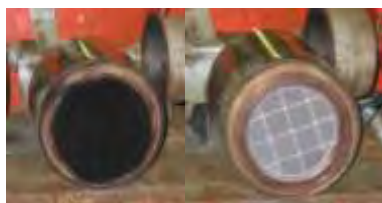
Figure 2: Entrapment of soot at inlet of filter
