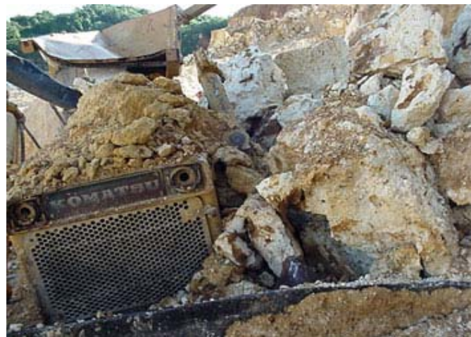
Figure 1 Highwall failure at a stone operation crushed this dozer, fatally injuring the operator (November 2002). Photograph courtesy of the Mine Safety and Health Administration.
