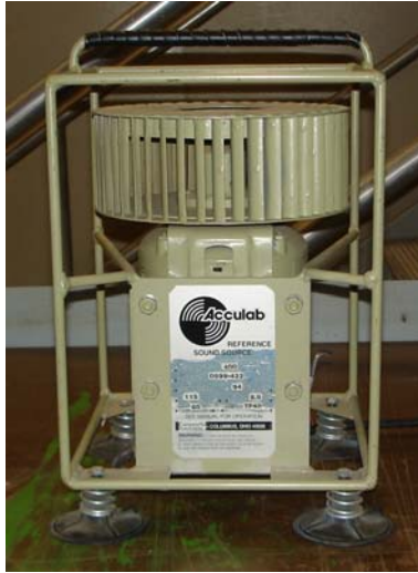
Figure 3: Calibrated Noise Source for Underground Testing
