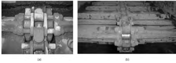
Fig. 1—CMM prototype dual sprocket chain (a) at the front foot shaft and single sprocket chain (b) at the rear tail roller.
