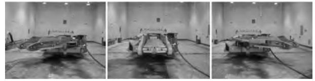
Fig. 4—CMM conveyor configurations: left, straight, right.
