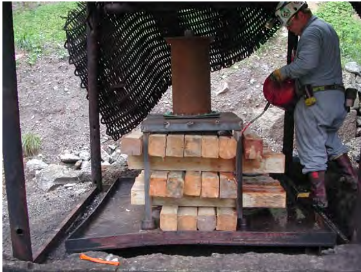
Figure 3. A USBM technician prepares to conduct a test that would eventually become Test 8(d) in the UN Test Manual. If the 45.3 kg (100 lb) of blasting agent loaded explodes when subjected to the fire it will not be approved for bulk transport.
