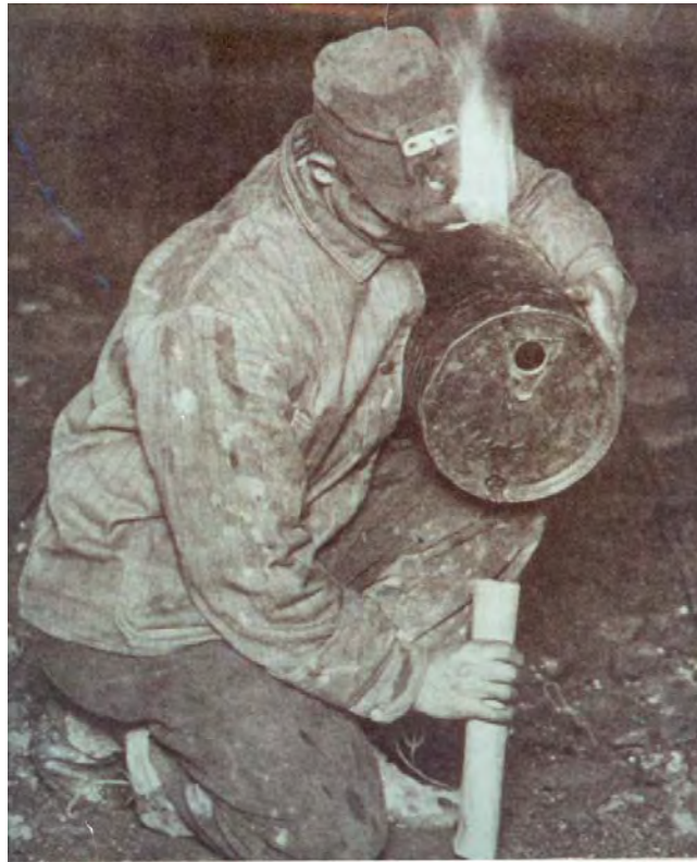
Figure 1. Miner making black powder cartridge for blasting coal.
