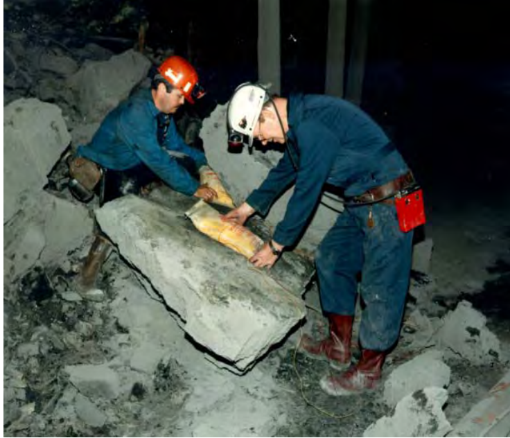
Figure 2. A miner and an explosives company technical representative preparing to break rock using the commercial version of the sheathed explosive charge, the Rock-Buster.
