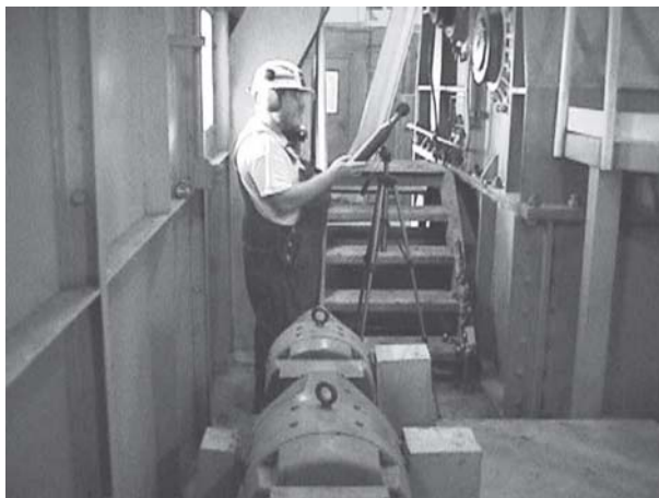
Figure 2 — Example of noise measurement at a worker location.
