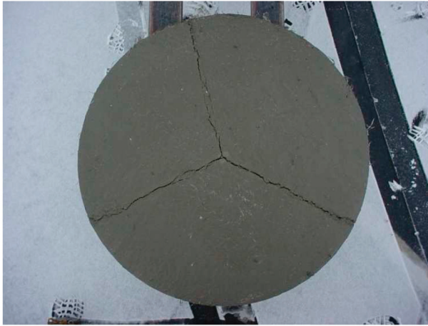
Figure 9 — Typical round panel with three cracks.
