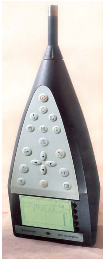
Figure 6.11 Photograph of a Brüel and Kjær 2260 Investigator
