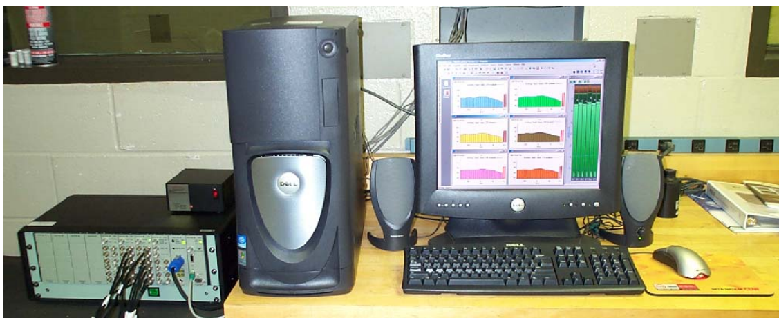
Figure 4.7. Bruel & Kjaer Pulse Data Acquisition System
