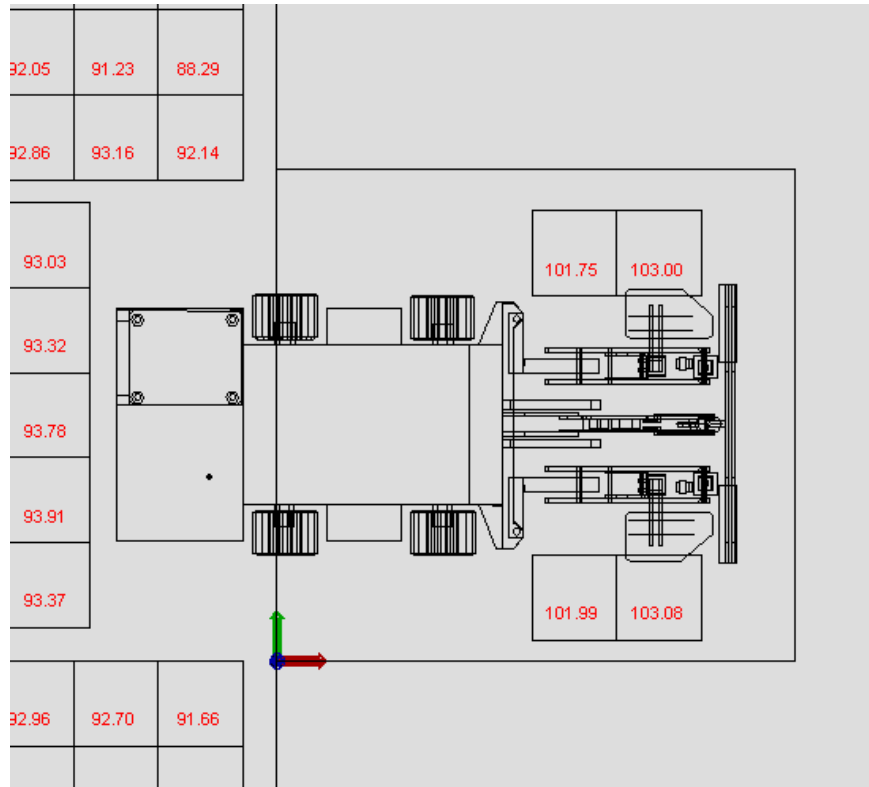
Figure 6.40 Zoom-view of Determined Sound Pressure Levels Near a Roof Bolting Machine
