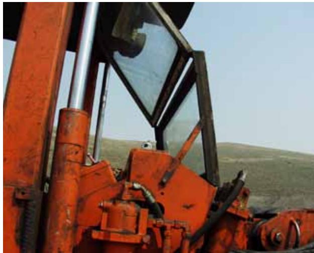
Figure 29. Windshield installed on bolter 2.
