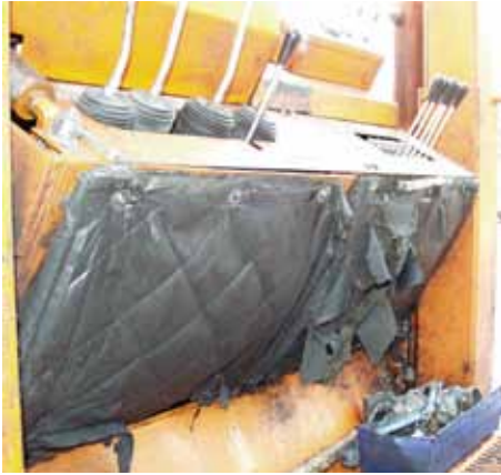
Figure 28. Quilted fiberglass material in the lower front of the operator's area of bolter 2.
