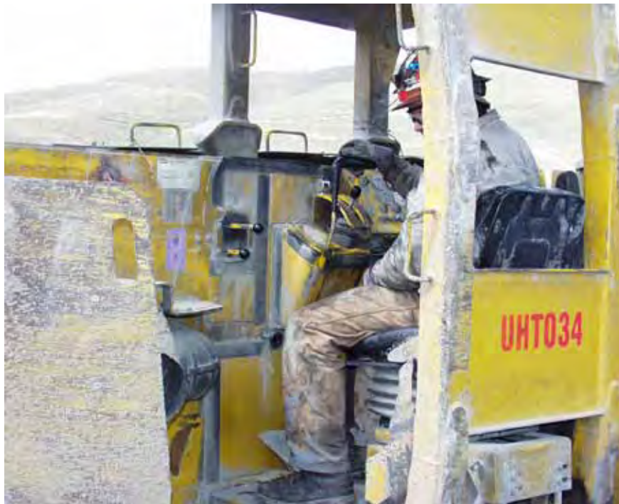
Figure 2. Haul truck without vinyl-covered material.
