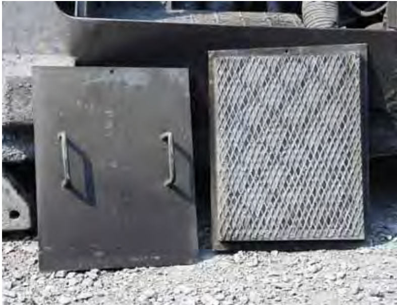
Figure 12. Front and back of the steel panels insulated with 1.5-inch-thick fiberglass.
