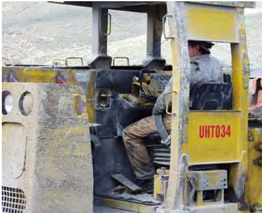
Figure 1. Haul truck with vinyl-covered material installed in the area in front of the operator.
