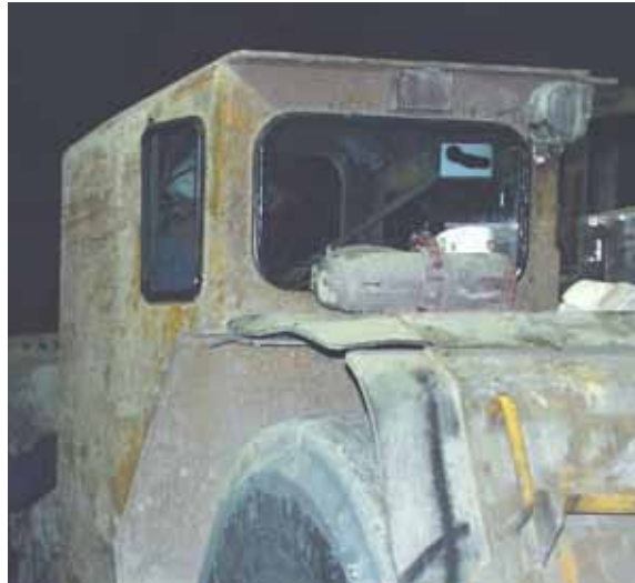
Figure 21. Enclosed cab with glass in place.
