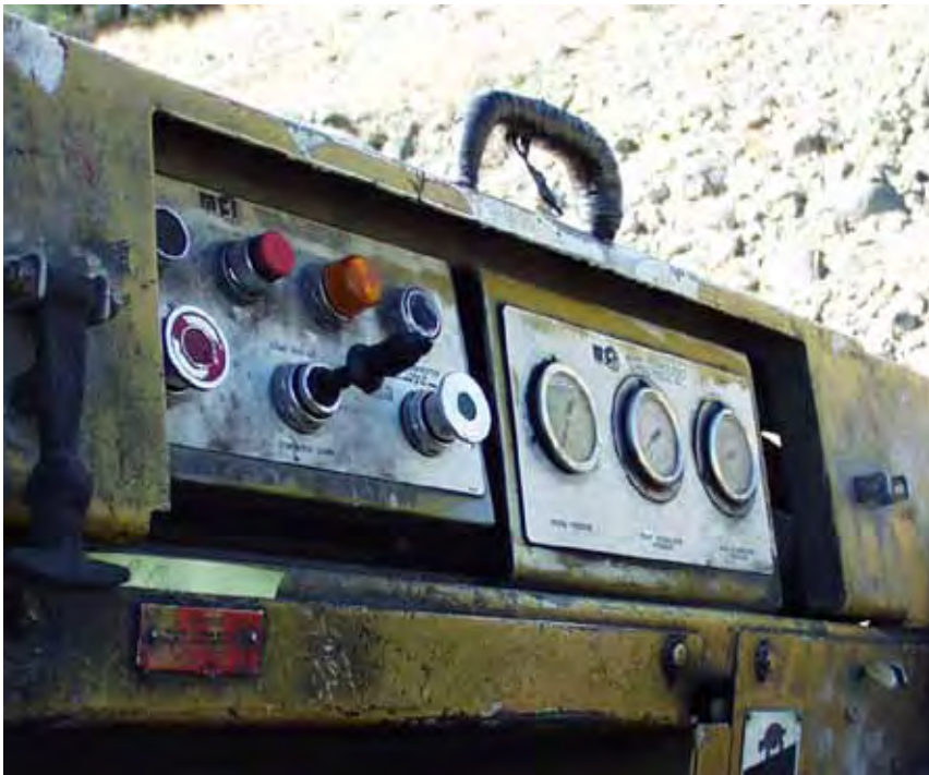
Figure 8. Direct openings to the engine compartment around instrument panel.
