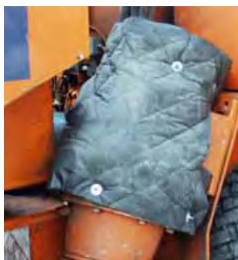
Figure 24. Fiberglass blanket barrier.
