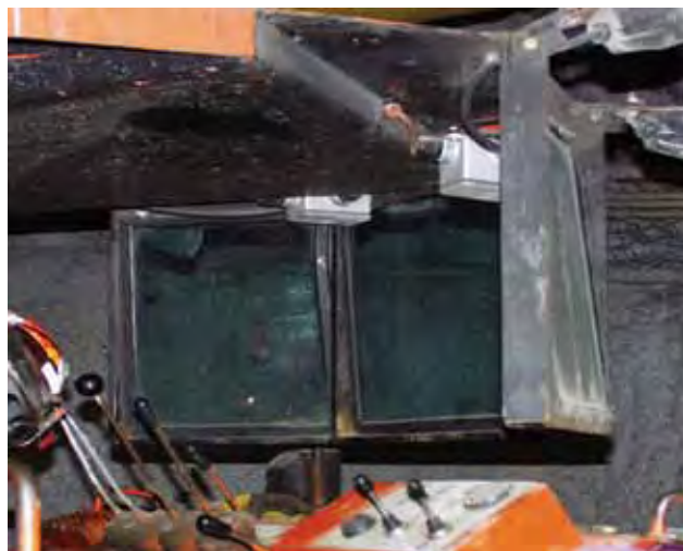
Figure 30. Windshield installed on bolter 3.
