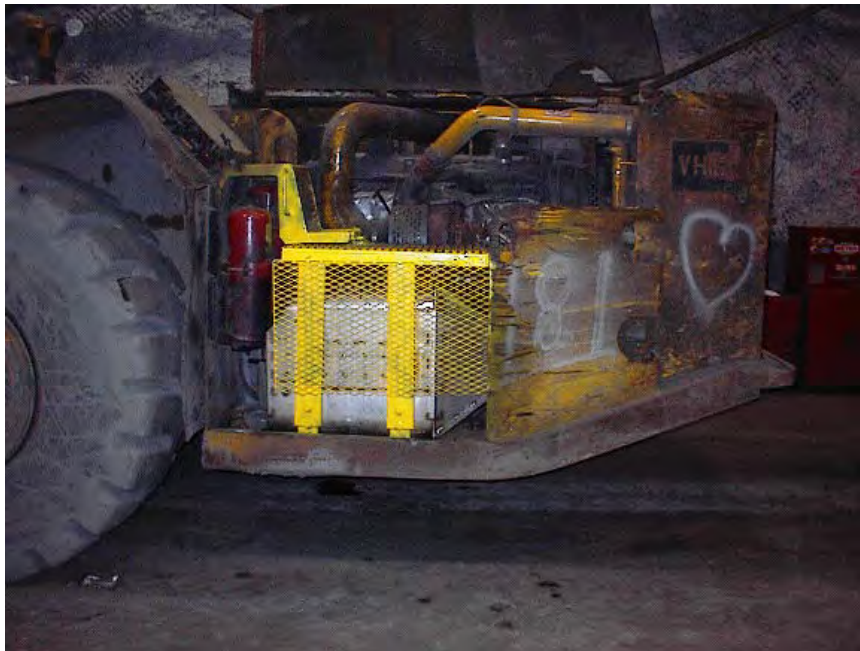
Figure 20 - Final Oberland Mangold DPF Installation
