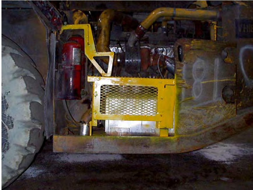
Figure 19 - Original Oberland Mangold DPF Installation
