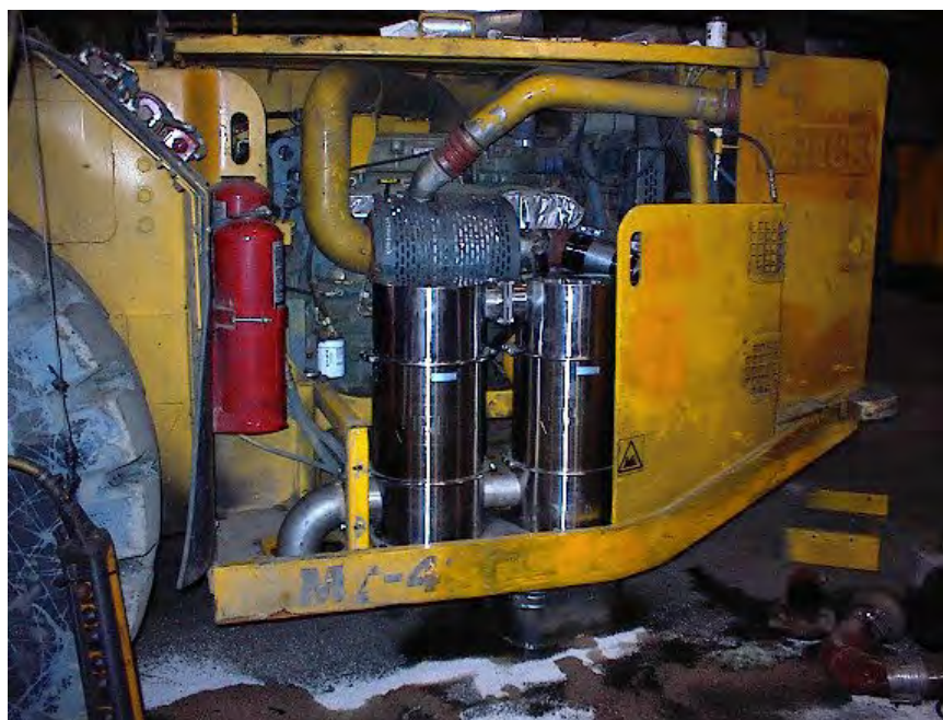
Figure 17 - ECS Octel Installation on VH183
