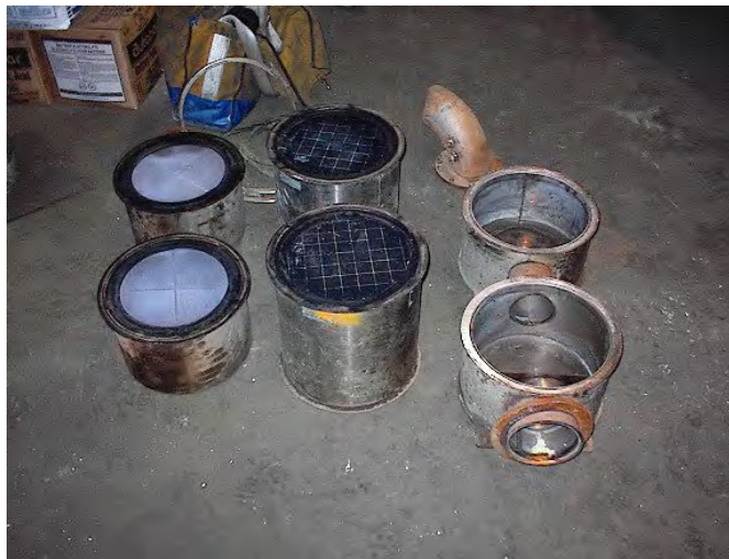
Figure 11 - ECS Octel DPF Components
