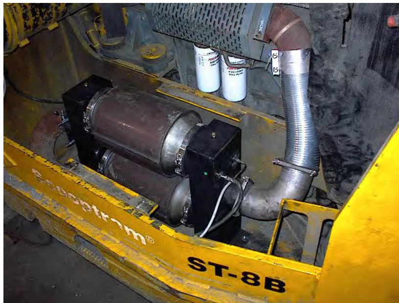
Figure 14 - ECS CatTrap Installation
