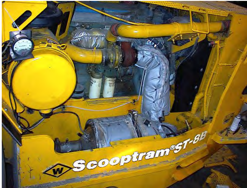
Figure 15 - DCL Bluesky Installation on VL247
