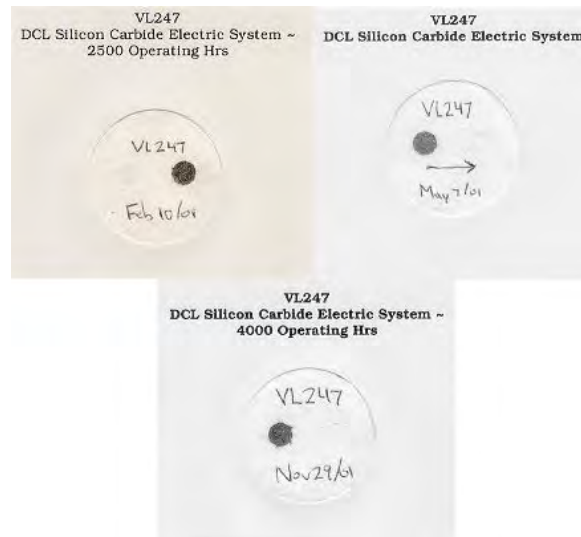
Figure 30 – Bacharach Smoke Density Results on VL247 with DCL Bluseky DPF System
