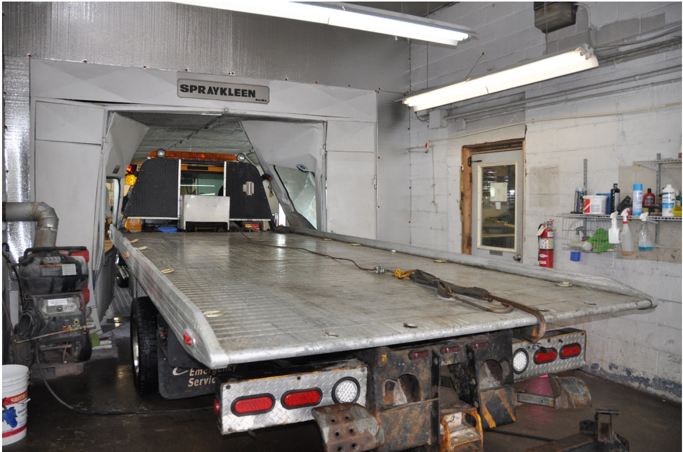
Photo 1. The Ford 550 Super Duty truck suddenly rolled forward 16 feet and crashed into the paint booth when the victim was cleaning the truck in the wash bay (photo courtesy of OSHA).
