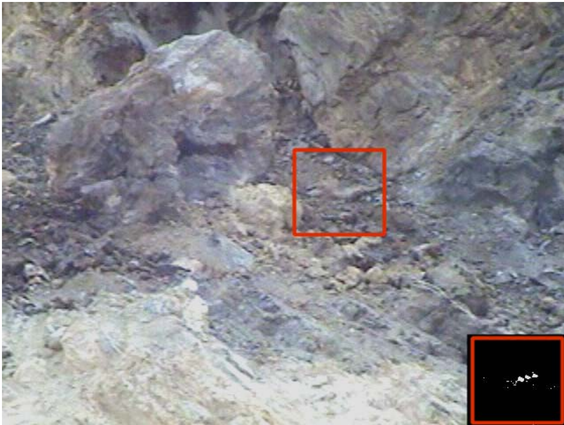
Figure 5.—Video frame captured during detection of a rockfall. Box shows where rock impact was detected. Inset shows where in the box differencing with a previous frame revealed changed pixels.
