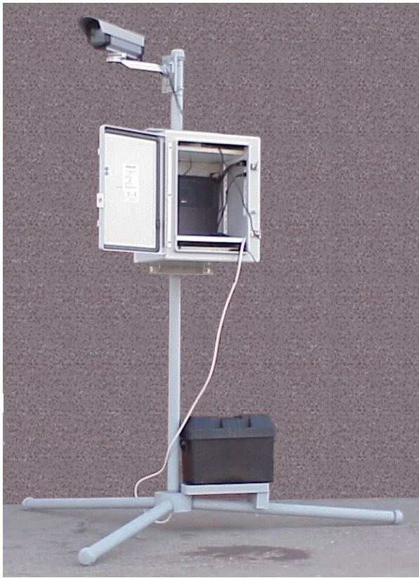
Figure 1.—Video motion-detection system showing camera, electronics enclosure, and 12-V battery on a tripod.
