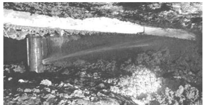
Figure 5 — Spray nozzle directing material towards mine rib (Gray et al., 2006).
