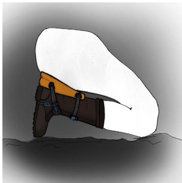
Fig. 2. A body weight support device worn at the ankle that reduces the flexion angle at the knee and increases the distribution of upper body weight through the heels.
