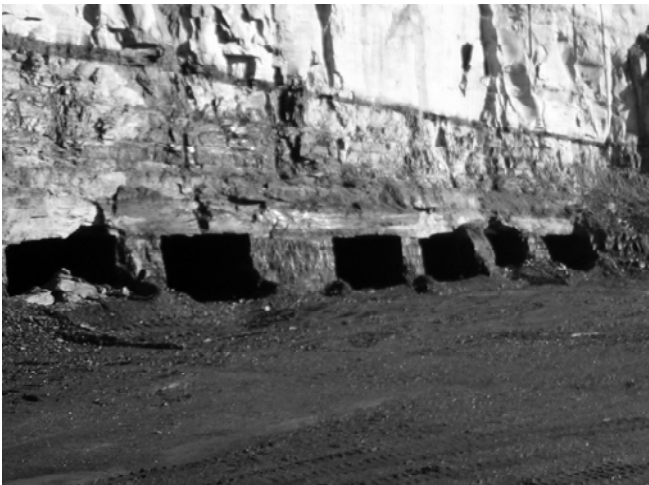
Figure 8. Typical highwall mining web and barrier pillars.
