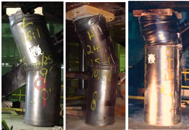
Figure 10. Buckling of Can caused by welding of sections together can create a hinge point during lateral displacement that may cause load shedding during yielding.
