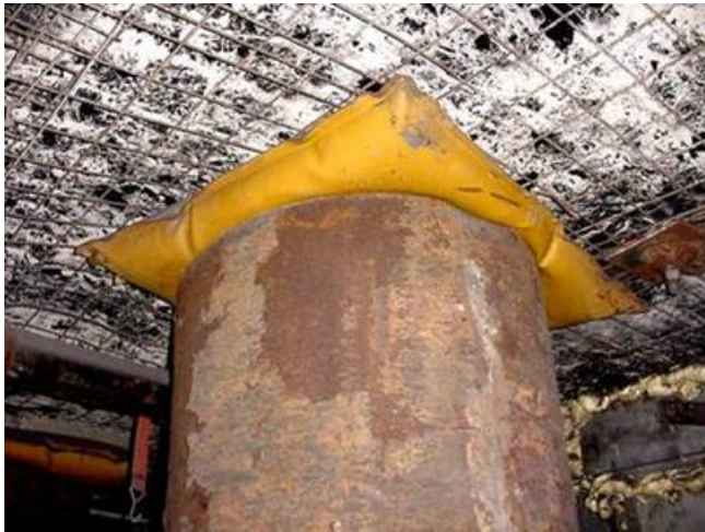
Figure 8. A water-filled prestressing unit (PSU) is now available for topping off the CAN and applying a substantial active loading to the mine roof and floor.
