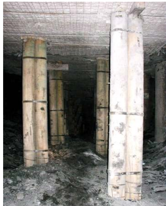
Figure 14. The Cluster Prop is three Wedge Props bundled together as shown in this longwall gateroad application.
