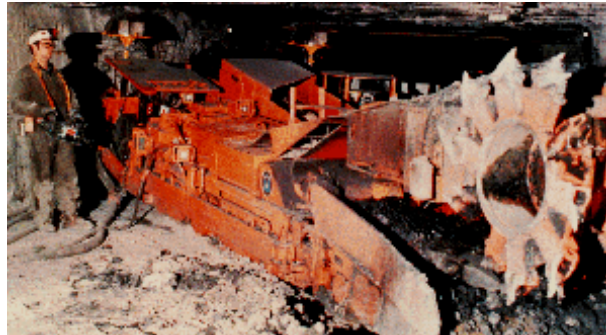
Figure 1.- Typical remote control continuous mining machine and its operator.
