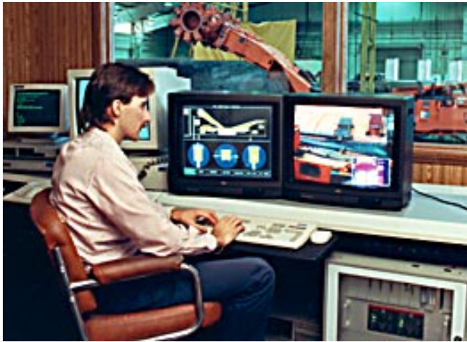
Computer-assisted mining systems allow the relocation of workers from the hazardous mineral extraction area to a safe, protected location.
