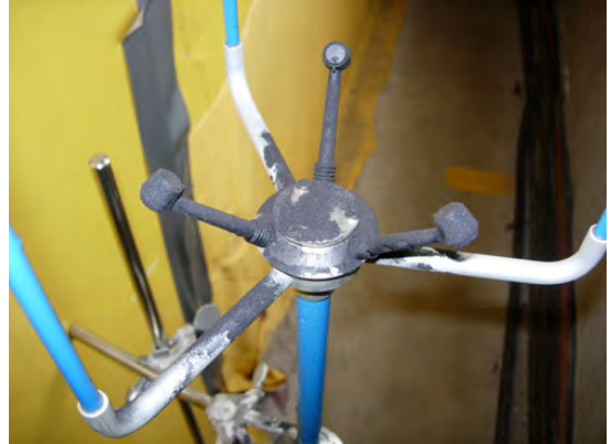
Figure 6 Wetted coal dust on 2-axis and 3-axis ultrasonic anemometer heads
