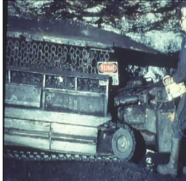
Figure 6. A Mobile Roof Support.
