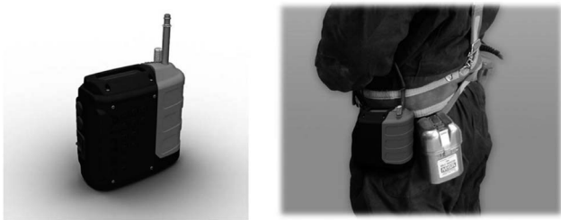
Fig. 1 Picture of the Airtec, the commercial version of the real-time EC monitor.
