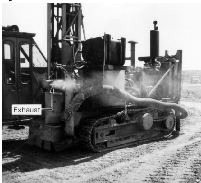
Visible dust in the Rotoclone exhaust of a coal mine drill.
