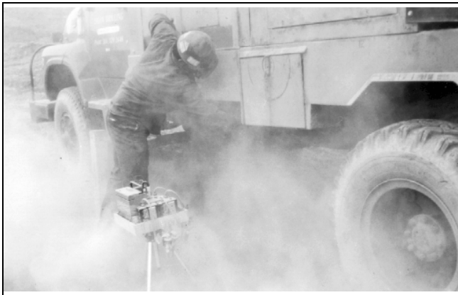
Dust cloud generated during Rotoclone dust collector dumping.
