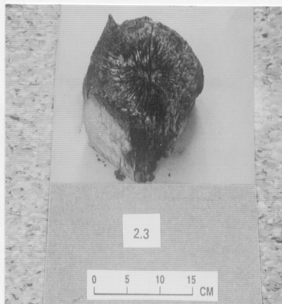
Figure 2.—Sample 2.3 (partially charred wood-crib block) from set 2.
